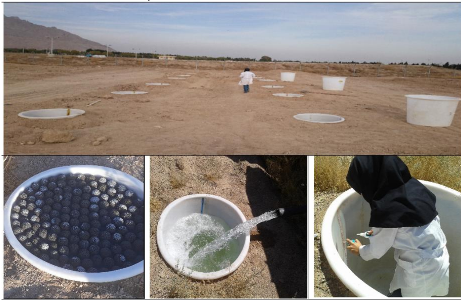
Figure 2- Steps for preparing tanks and placing concrete covers at Isfahan University of Technology site
