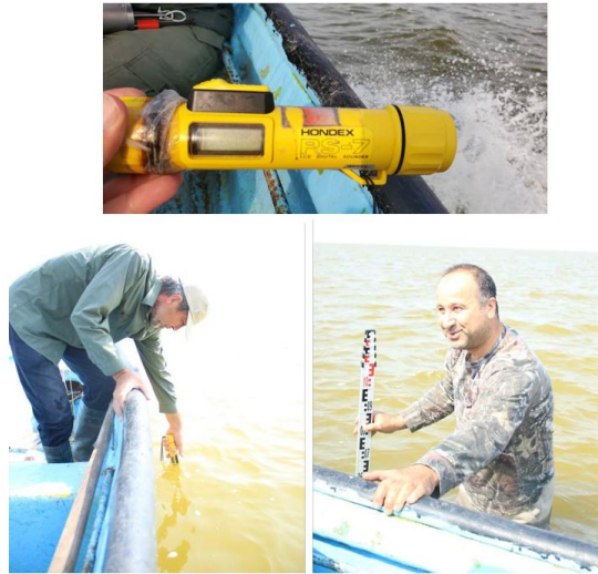
Figure 1: Depth measurement operation in the Gorgan Bay Wetland and Miankaleh.
